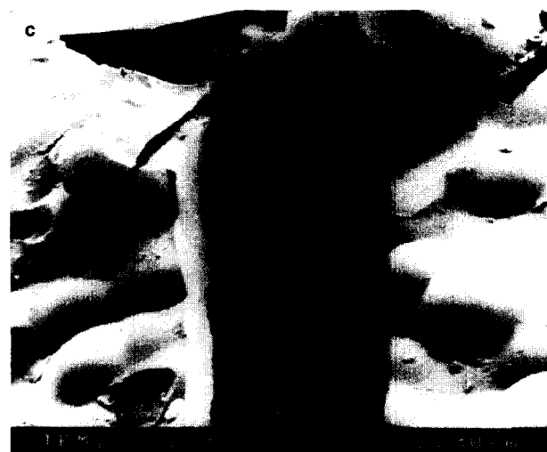
Figure 3 (a) A crack with a thin silica layer at its base (FEP) indicating, that the crack has been formed during the hydrolysis in the autoclave. (b) Cracked surface formed during sample preparation used for estimating the thickness of the silica layer (TFM). (c) Fibrils pulled out of the polymer surface (TFM) indicating adhesion between the silica and the perfluorinated polymer
