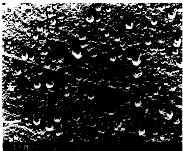
Figure 1 (a) Untreated polymer surface (TFM), representative for all three polymer types, modified in this work. (b) A survey of a silica covered polymer surface (TFM). All samples, shown as micrographs, were treated at 125°C for 40 h. The pressure of the water vapour was 800 kPa. The treatment conditions are as described in the experiment part
